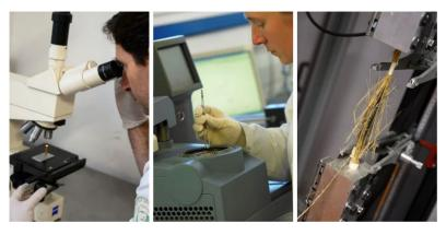
Type testing is undertaken to **ASTM B987** with certification provided on different core sizes for both **HVCRC**® and **HVCRC**®ULS (Extra High Strength Grade).
